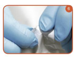
6. Tear the aluminium envelope open at the notch. Once the device has been taken out of the envelope its stability is of short duration, especially in a humid environment.
