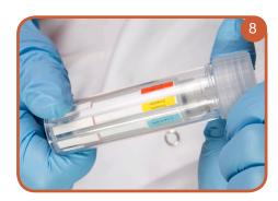
Screw the top of the strip tube. You must hear two separate clicks, for perforation of superior and inferior septa of the sample tube. Leave the device vertically on a flat surface and wait for 10 minutes. The liquid contained in the sample tube moves to the strip tube and slowly migrates along the strips.
