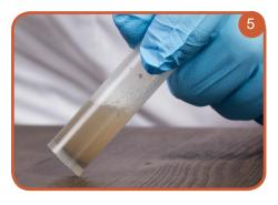
5. Tap the sample tube on a hard surface so that all the liquid is collected at the bottom of the tube.
