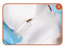
3. Dilute its content in the liquid of the small tube called sample tube.
