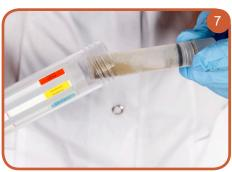
7. Insert the sample tube into the strip tube.
